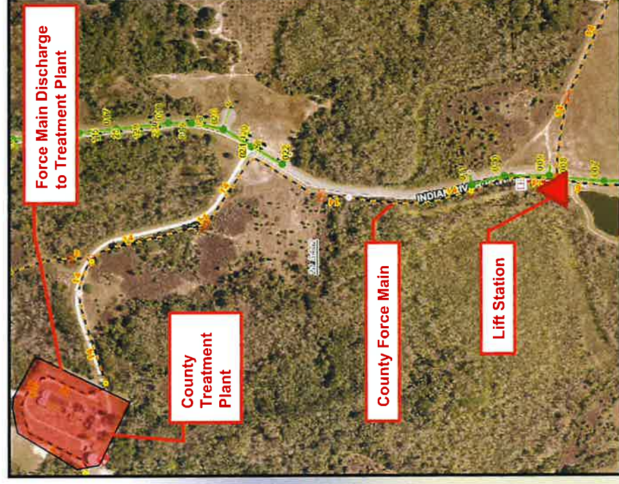
Figure 7 – Typical Force Main Discharge to Treatment Plant
