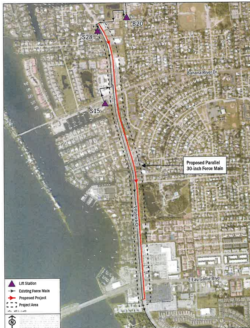
Figure 5-1. Proposed Wastewater Improvements
