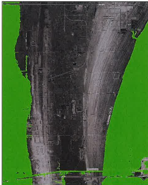
Figure 3.1: Missing Topographic Information
