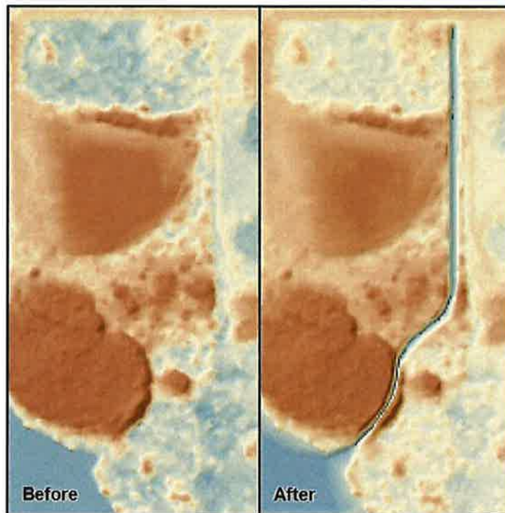
Figure 3.8: Corrected Topographic Void of New Channel Excavation
